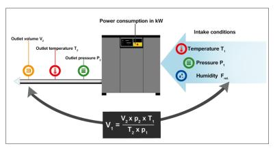
The delivery rate of compressors depends on the intake air.
