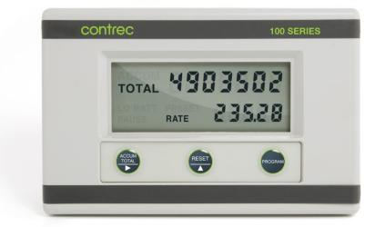
The 104D is a 4-20mA Loop Powered Rate Totaliser and is designed to operate with Turbine, Positive Displacement and Paddlewheel Flowmeters in applications such as irrigation systems and pipelines, and as a replacement for mechanical registers.
