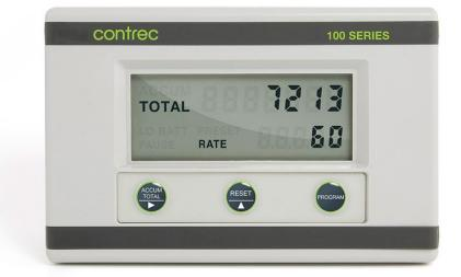
The 102A Rate Totaliser is designed to operate with any flowmeter which produces a 4-20mA output, including Differential Pressure Devices, Magnetic or Vortex Flowmeters. The unit is powered entirely from the 4-20mA current loop.
